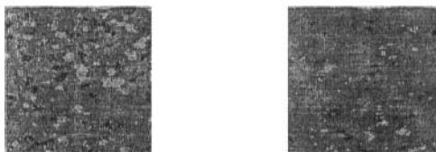
FIGURE3 Change in the atomic force microscopy of DOCDA-DAP polyimide; (left) after modification (right) after LP-UV light irradiation.
